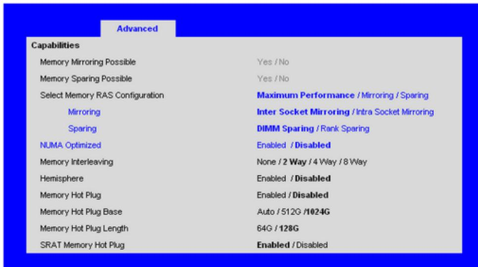
**Figure 6-5** Setup Utility—Configure Memory and RAS and Performance Screen
