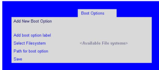
**Figure 6-17** Setup Utility—Add New Boot Option Screen
