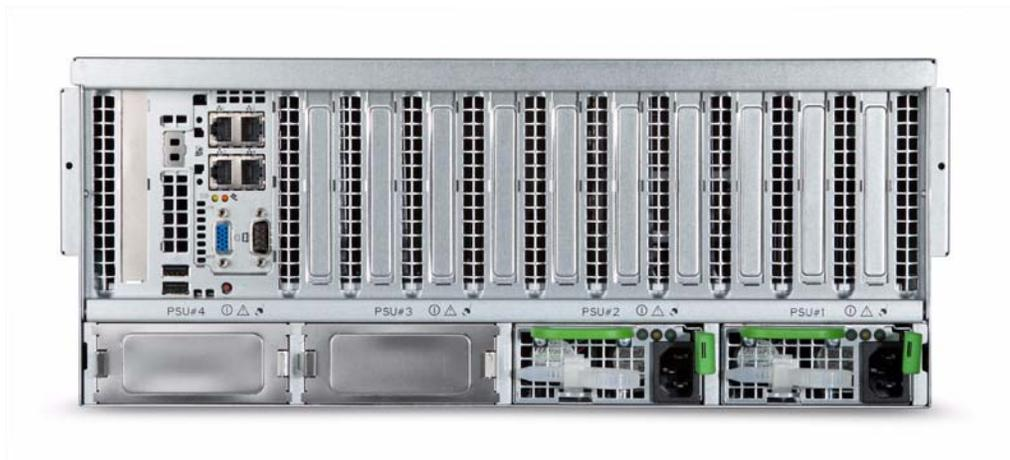
**Figure 1-6** SGI Altix UV 10 Rear View
