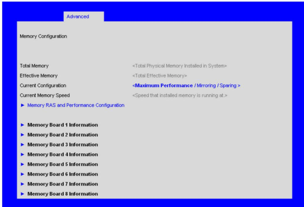
**Figure 6-4** Setup Utility—Memory Configuration Screen
