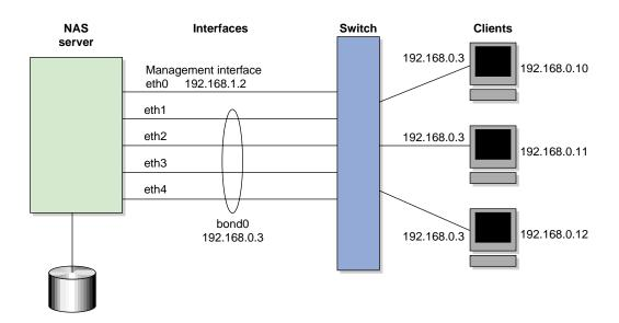
Figure 3-3 Bonded Network Interfaces
