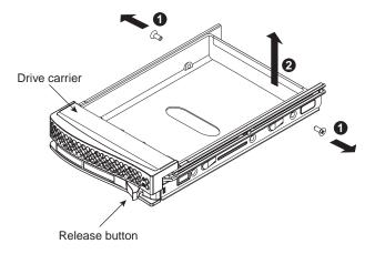
**Figure 4-2** Removing the Dummy Drive from the Carrier
