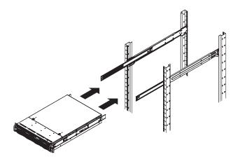
Figure 3-5 Installing the Server in a Rack
