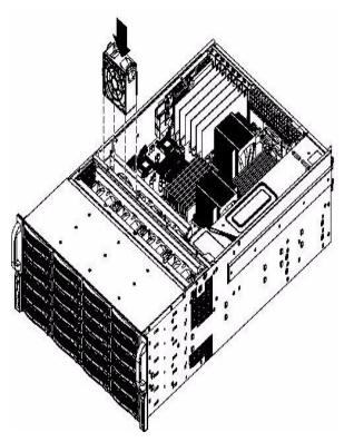
Figure 4-6 Replacing a Fan
