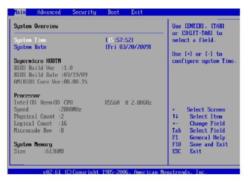
Figure 6-1 System Overview Main BIOS Setup Screen
