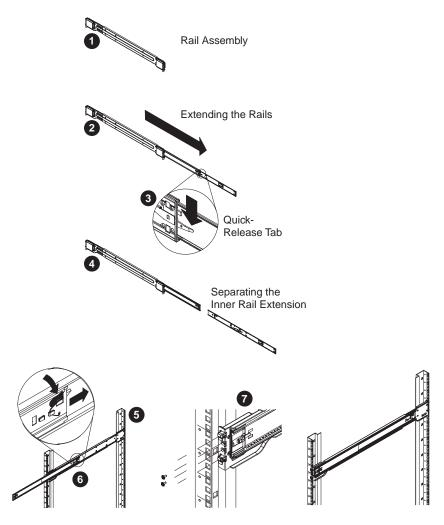
Figure 3-1 Separating and Installing the Rack Rails
