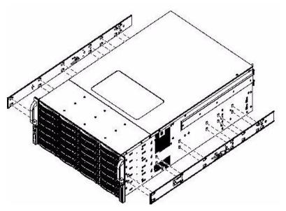
Figure 3-4 Installing the Inner Rail Extensions
