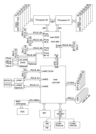
Figure 1-2 ISS3500 Serverboard Block Diagram
