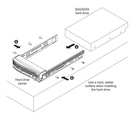
Figure 4-3 Installing a Drive into a Hard Drive Carrier
