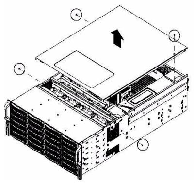
Figure 3-6 Removing the Chassis Cover
