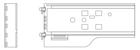
Figure 3-2 Square-to-round Hole Adapter for 2U Quick Attach Rails
