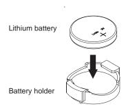
Figure 2-1 Installing the Onboard Battery
