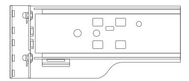
Figure 3-3 Square-to-round Hole Adapter Clipped onto the Rail Set
