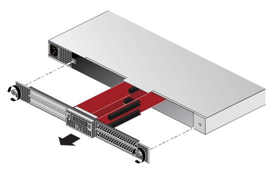
Figure 5-3 Card Slot Locations in "PCIe Carriage"
