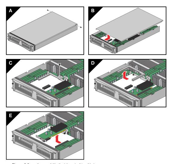
**Figure 5-5** Remove PCIe Card from the Riser Blade
