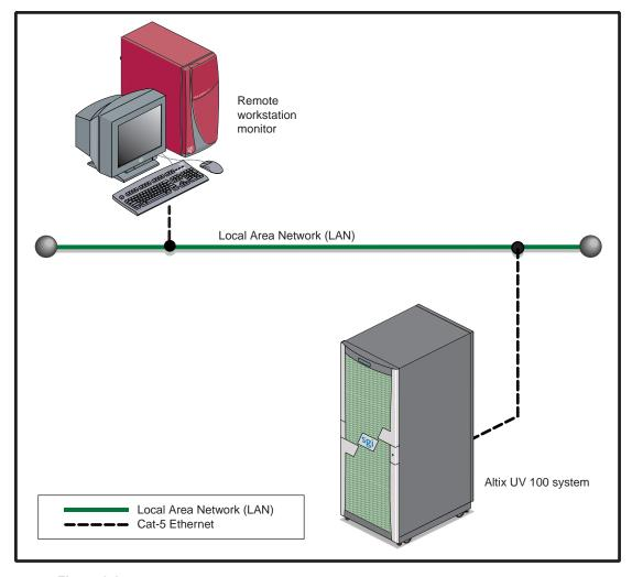
Figure 2-2 SGI Altix UV 100 LAN-attached System Control Network
