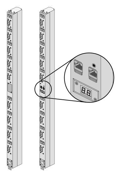
Figure 1-6 Three-Phase PDU Examples
