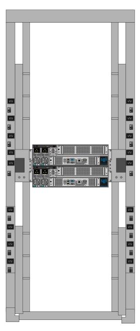
Figure 3-2 SGI Altix UV 100 IRU and Rack Example
