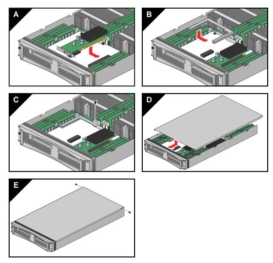
Figure 5-6 Replace PCIe Card
