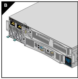
Figure 5-7 Reinstall PCIe Riser Blade in the UV 100
