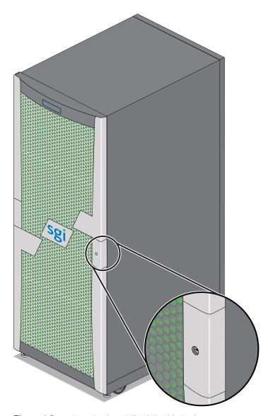
Figure 4-5 Front Lock on Tall (42U) Altix Rack
