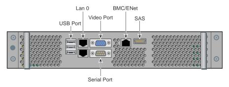
Figure 3-7 BaseIO Riser Enabled Blade Front Panel Example
