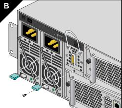
Figure 5-12 Replace the Disk Drive Tray
