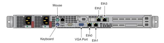
Figure 2-4 Optional System Management Node (SMN) Direct Video Connection Ports
