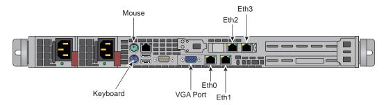
Figure 1-1 Optional System Management Node VGA Connection Points
