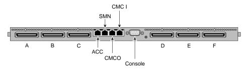
Figure 1-2 UV 100 CMC Connections
