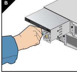
Figure 5-9 UV 100 Drive Tray Removal
