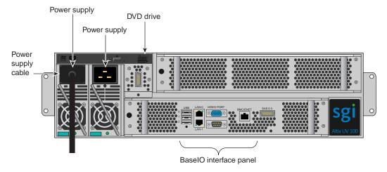
**Figure 1-3** IRU Power Supply Cable Location Example
