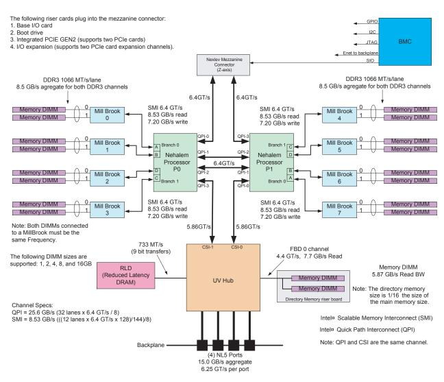
Figure 3-4 Blade Node Block Diagram
