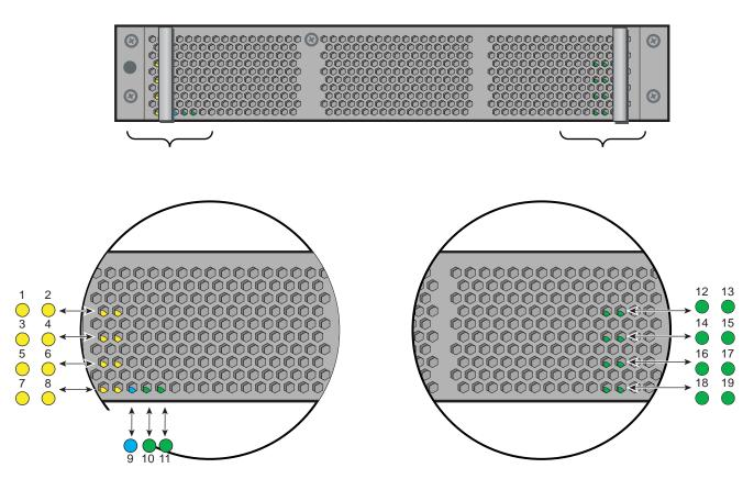
Figure 6-1 UV Compute Blade Status LED Locations
