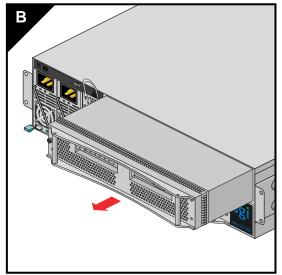
**Figure 5-4** Extracting the PCIe Riser Blade From the Enclosure
