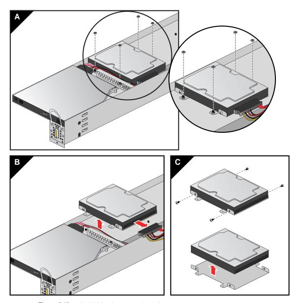
Figure 5-10 Hard Disk Drive Remove Example
