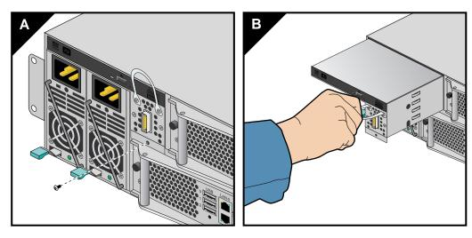
Figure 5-13 UV 100 Drive Tray Removal
