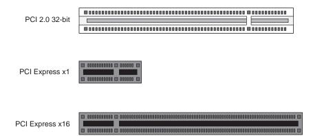
Figure 5-1 Comparison of PCI/PCI-X Connector with PCI Express Connectors
