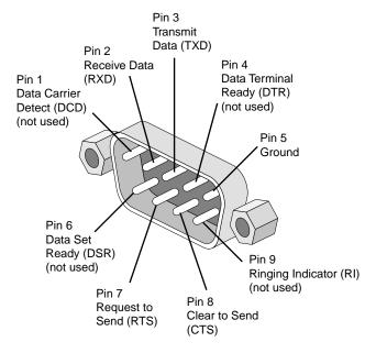
Figure A-2 Serial Port Connector
