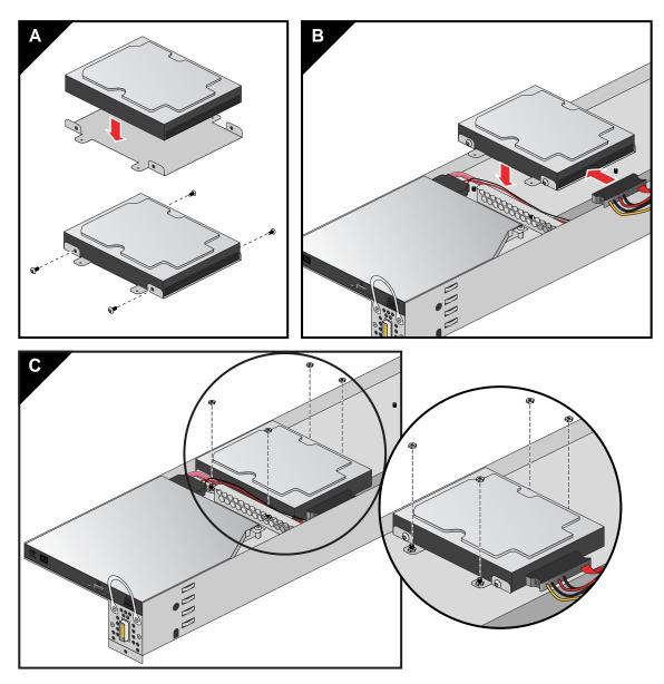
Figure 5-11 Install New Disk Drive Example
