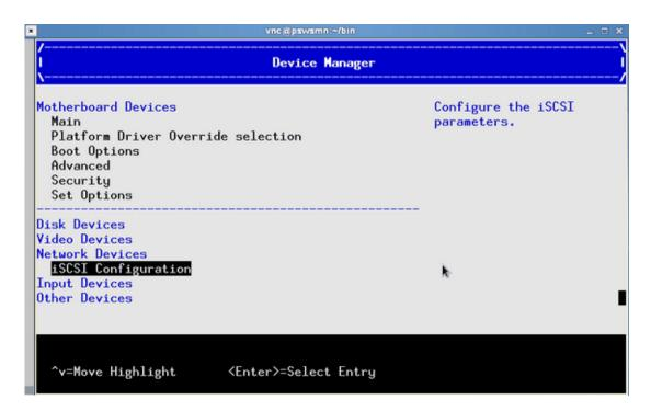
Figure 2-11 Device Manager iSCSI Configuration Screen
