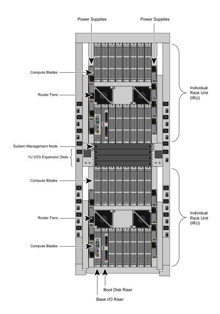
Figure 1-1 SGI Altix UV 1000 System Rack
