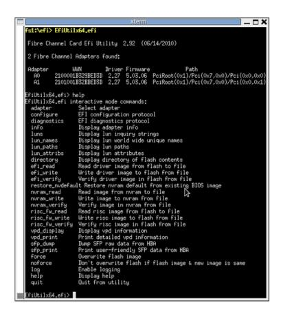
Figure 3-10 Fibre Channel Card EFI Utility (EFIUtilx64.efi)
