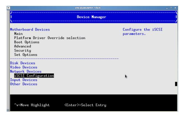
Figure 3-1 Device Manager iSCSI Configuration Screen
