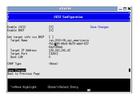
Figure 3-5 iSCSI Configuration 4 of 4 Screen
