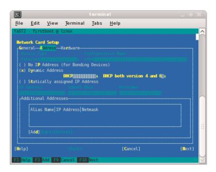
Figure 1-7 Network Card Setup Screen
