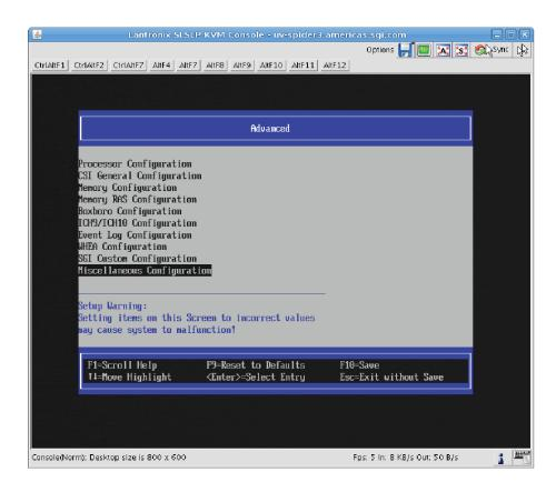
Figure 2-5 Advanced Boot Setup Screen
