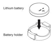
Figure 4-1 Installing the Onboard Battery
