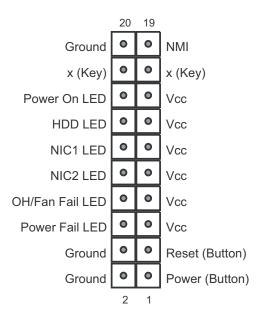
Figure 5-1 Control Panel Header Pins
