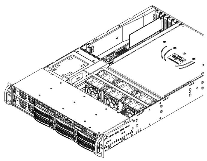
Figure 6-1 System Cooling Fan Locations
