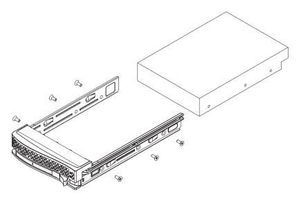
**Figure 6-2** Mounting a Drive in a Carrier
