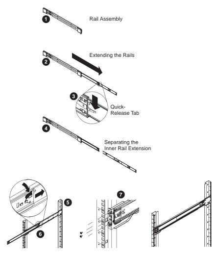
Figure 2-1 Separating and Installing the Rack Rails
