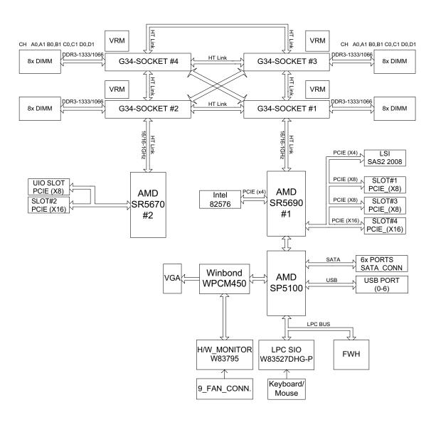
Figure 1-2 Processor and I/O Chipset System Block Diagram
