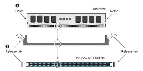
Figure 5-4 DIMM Installation Example
