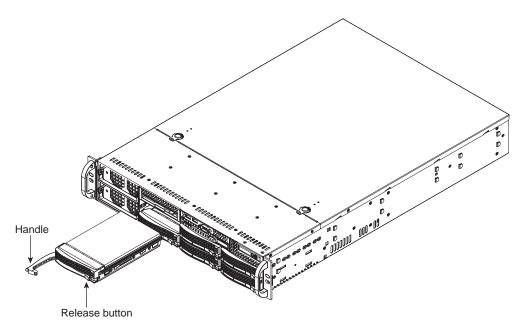
Figure 6-3 Removing a Disk Drive Carrier
