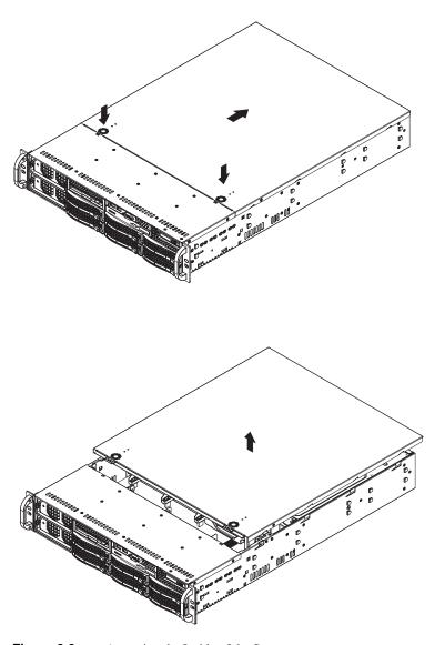
Figure 2-3 Accessing the Inside of the System
