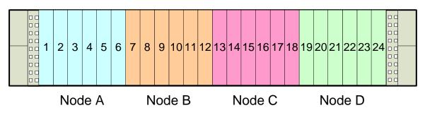
Figure 6-3 Disk Drives and Associated Nodes in the 24-Drive Configuration
