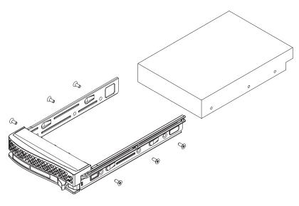
Figure 6-4 Mounting a Drive in a Carrier
