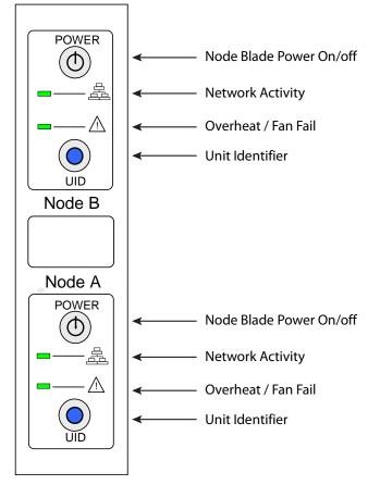
Figure 3-2 Control Panel Buttons and LEDs
