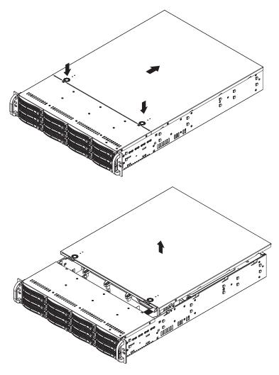
Figure 2-3 Accessing the Inside of the System
