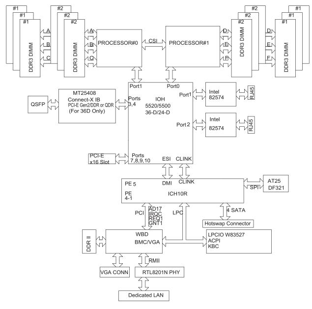
Figure 1-2 Intel 5520 Chipset—System Block Diagram
