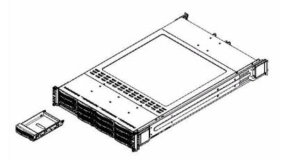
Figure 6-5Removing a Drive Carrier
