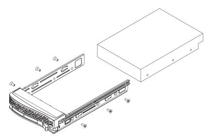
Figure 6-4 Mounting a Drive in a Carrier
