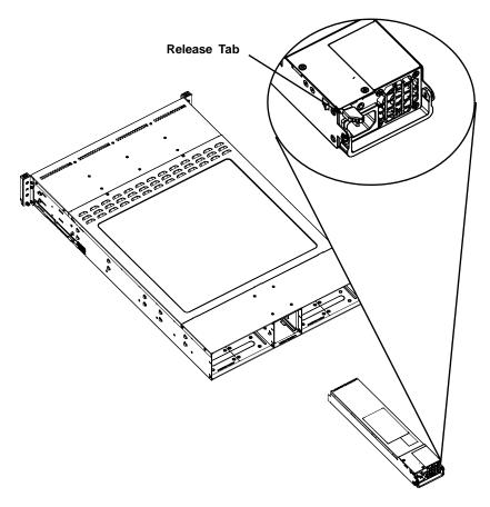
Figure 6-6 Removing a Power Supply
