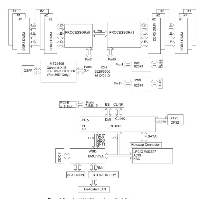
Figure 1-2 Intel 5520 Chipset—System Block Diagram
