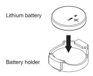
Figure 4-1 Installing the Onboard Battery
