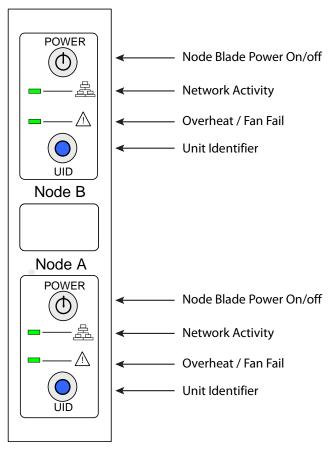
Figure 3-2 Control Panel Buttons and LEDs
