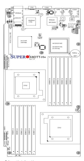
Figure 5-1 Node Board Layout
