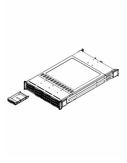
Figure 6-5 Removing a Drive Carrier
