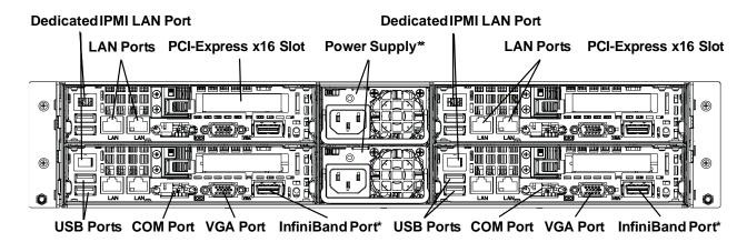
Figure 5-2 Serverboard I/O Ports
