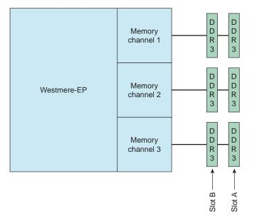
Figure 5-3 Memory Block Diagram
