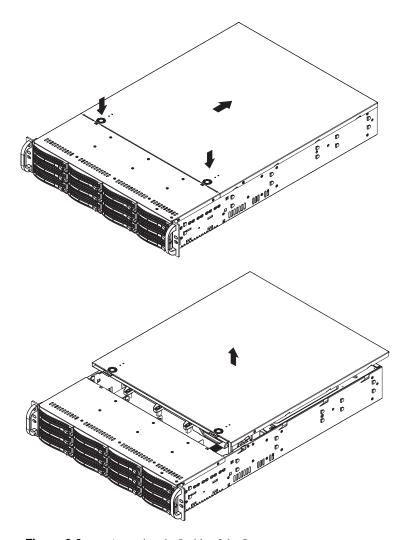
Figure 2-3 Accessing the Inside of the System
