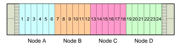
Figure 6-3 Disk Drives and Associated Nodes in the 24-Drive Configuration
