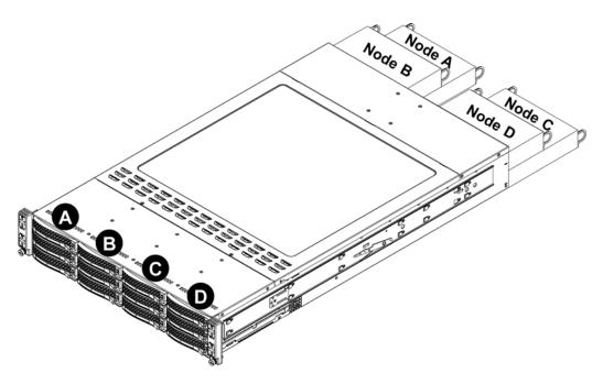
Figure 6-2 Disk Drives and Associated Nodes in the 12-Drive Configuration
