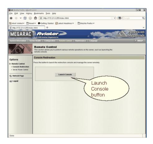
Figure 3-4 BMC Remote Control Console Redirection Screen
