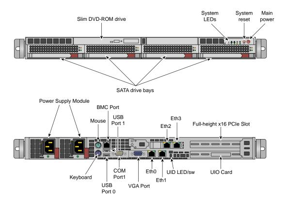
Figure 1-1 System Management Node Front and Rear Panels
