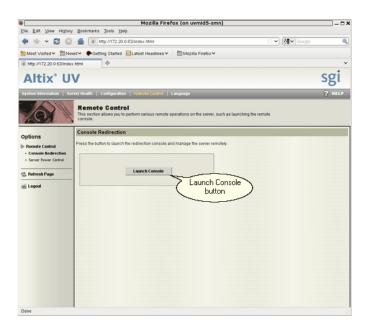
Figure 3-4 BMC Remote Control Console Redirection Screen
