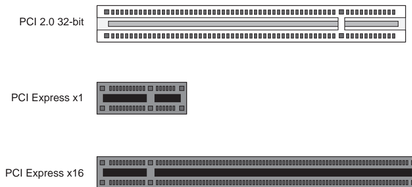
Figure 7-5 Comparison of PCI/PCI-X Connector with PCI Express Connectors
