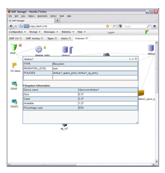
Figure 2-3 User Filesystem Capacity in DMF Manager
