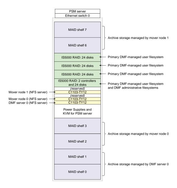
Figure 1-1 ArcFiniti Components
