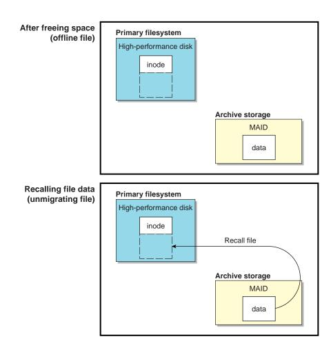
Figure 1-3 Freeing and Recalling File Data
