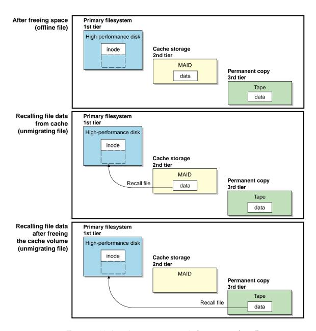
Figure 1-6 COPAN MAID as a Fast-Mount Cache: Freeing and Recalling Data
