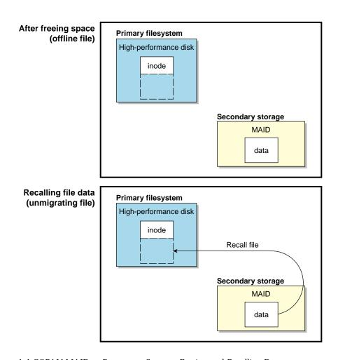
Figure 1-4 COPAN MAID as Permanent Storage: Freeing and Recalling Data
