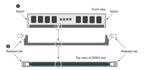
Figure 5-4 DIMM Installation Example
