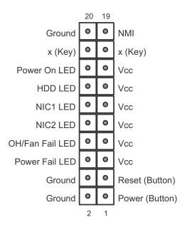
Figure 5-1 Control Panel Header Pins
