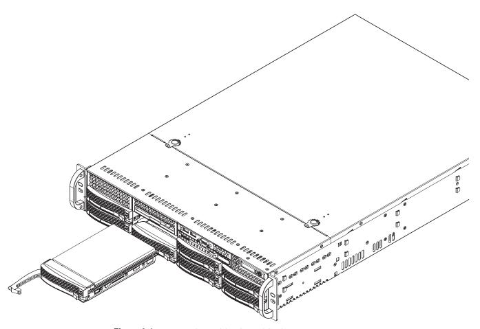
Figure 6-4 Removing a Disk Drive and Carrier
