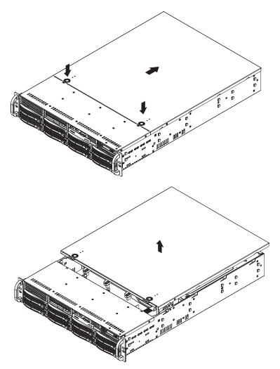
Figure 2-4 Accessing the Inside of the System
