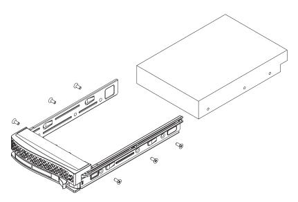
Figure 6-3 Mounting a Drive in a Carrier
