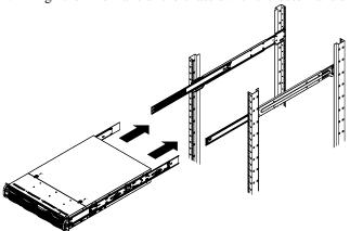
Figure 2-3 Installing the Server in the Rack
