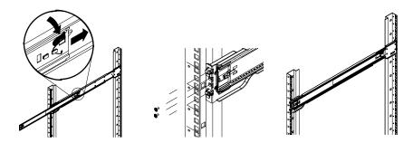
Figure 2-2 Outer Rack Rail Assembly Example
