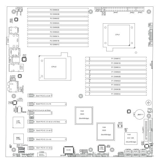
Figure 5-2 Node Board Layout
