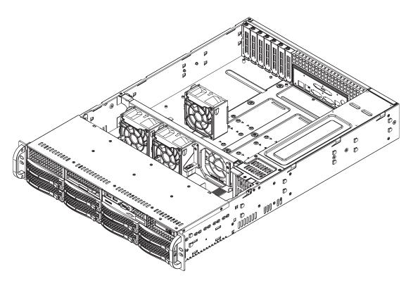
**Figure 6-3** Removing System Cooling Fans
