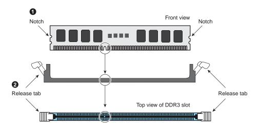
Figure 5-3 DIMM Installation
