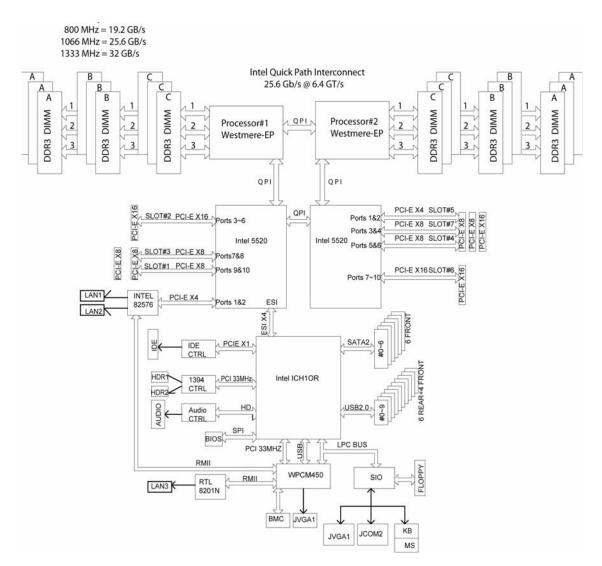
Figure 1-2 Serverboard Block Diagram
