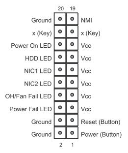
Figure 5-1 Control Panel Header Pins
