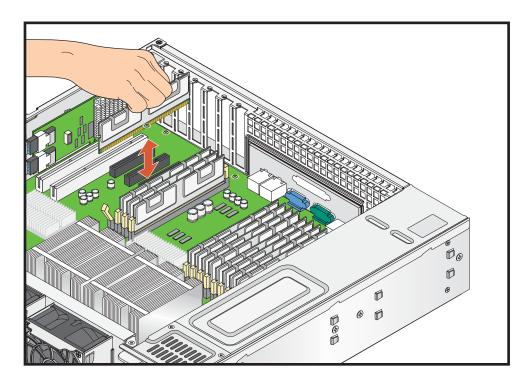
Figure 5-5 Removing a DIMM Module
