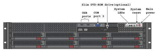
Figure 6-1 Front Chassis View
