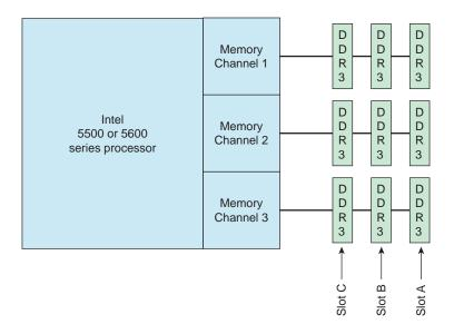
Figure 5-7 Memory Block Diagram
