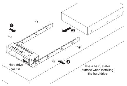
Figure 6-4 Mounting a Drive in a Carrier
