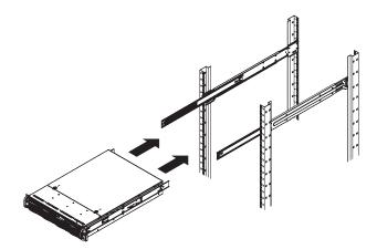
Figure 2-2 Installing the Server in a Rack
