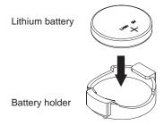
Figure 4-1 Installing the Onboard Battery
