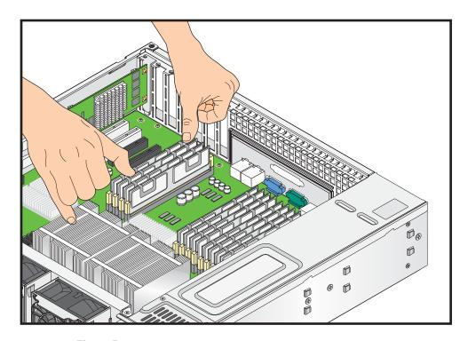
Figure 5-4 Installing DIMM Modules
