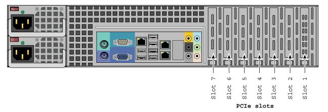
Figure 5-9 PCI Expansion Slots
