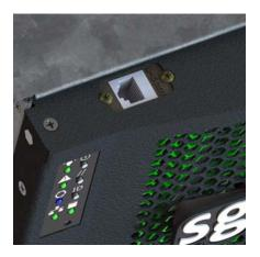
Figure 3-45 MIS-S9D proprietary network interface
