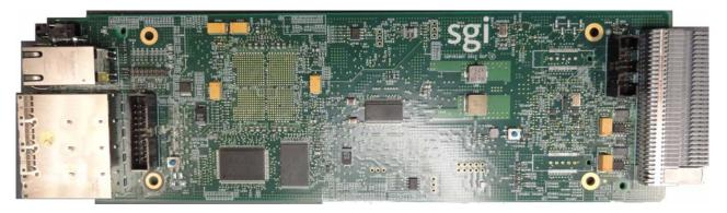
Figure 1-26 I/O Module for MIS JBOD Unit
