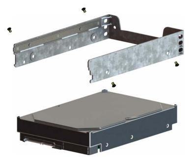
Figure 4-4 Hard Drive Carrier
