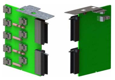
Figure 1-27 MIS JBOD Midplane I/O Connector (right & left views)
