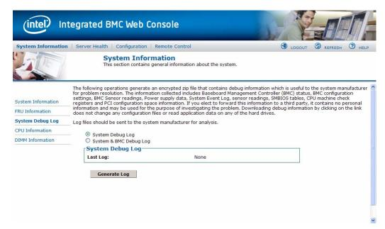
Figure 2-6 BMC Web Console – System Debug Log
