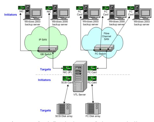
As you can see from the illustration above, an application server can be either an iSCSI client or a Fibre Channel client, but not both. Using separate cards and switches, you can have all types of COPAN 400 Clients (FC and iSCSI) on your network.
