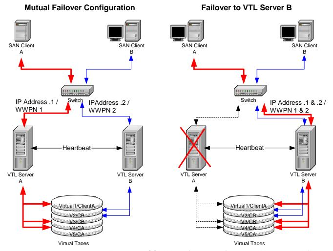
This diagram illustrates a COPAN 400 failover configuration. When server A fails, server B takes over and serves the clients of server A in addition to its own clients.
