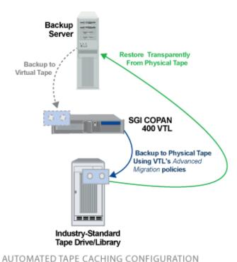
As in the Advanced COPAN 400 Configuration, backup software runs on a backup server and transparently manages the backup to virtual tape.
