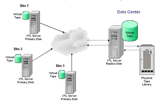
The following information is for environments with multiple COPAN 400 locations without physical tape libraries that replicate tape data to a remote COPAN 400 server that has a physical tape library that supports barcodes.
