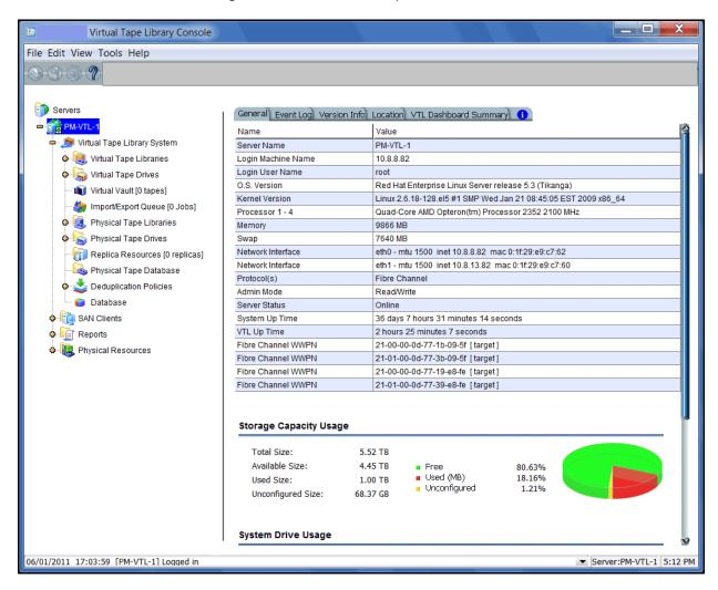
The tree allows you to navigate the various COPAN 400 appliances and their configuration objects. You can expand or collapse the display to show only the information that you wish to view. To expand a collapsed item, click the symbol next to the item. To collapse an item, click the symbol next to the item. Double-clicking on the item will also toggle the expanded/collapsed view of the item.
