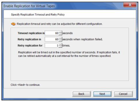
Replication can only occur when the virtual tape is not in a tape drive. Indicate how long the system should attempt to replicate data before timing out and how often it should attempt to retry before skipping a scheduled replication.
