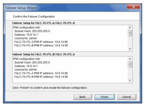
Once your configuration is complete, each time you connect to either server in the Console, you will automatically be connected to the other as well.
