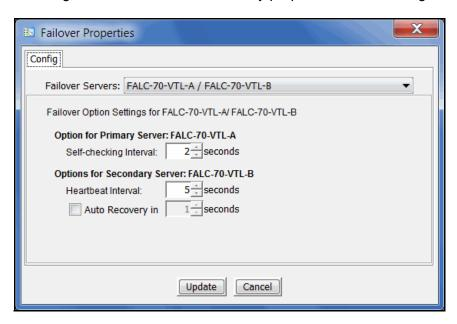
Note: We recommend keeping the Self-checking Interval and Heartbeat Interval set to the default values. Changing the values can result in a significantly longer failover and recovery process.
