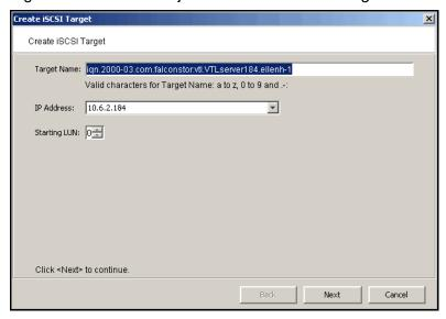
4. Enter a name for the target or accept the default and select the IP address of the adapter on the COPAN 400 server.
