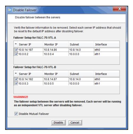
If everything is checked, as in the example above, this eliminates the failover relationship and removes the health monitoring IP addresses from the servers and restores the server IP addresses. If you uncheck the IP address(es) for a server, the health monitoring address becomes the server IP address.
