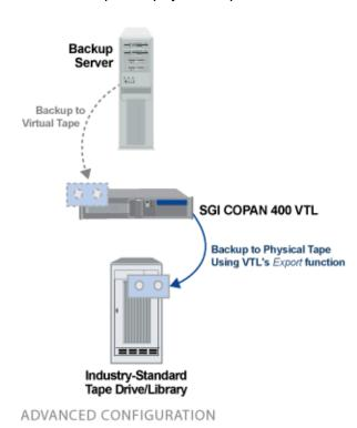
COPAN 400 dramatically accelerates backups by acting as a *defacto* cache to your physical tape library and enables data to be moved to physical tapes as a background process without impacting production servers. This is an innovative approach to backup that addresses the limitations of conventional tape backup. Moreover, since COPAN 400 manages the export of data from virtual to physical tapes, there is no additional overhead for the backup server.
