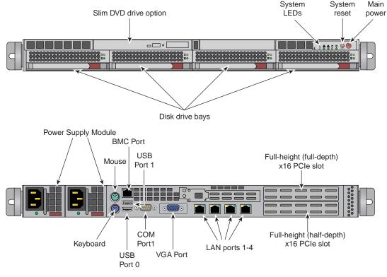
Figure 2-1 System Management Node Front and Rear Panels
