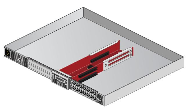
Figure 6-2The PCIe Expansion Enclosure
