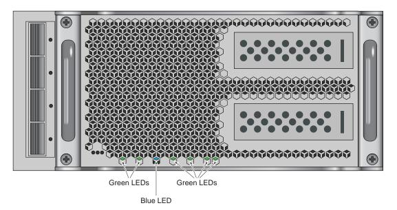
Figure 7-1 UV Compute Blade Status LED Locations Example
