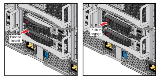
Figure 6-10 Replacing the UV 2000 System Disk Example
