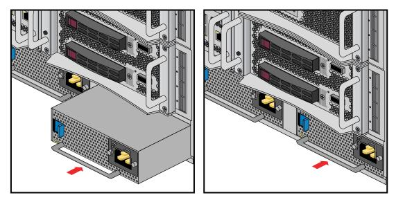
Figure 6-5Replacing an IRU Enclosure Power Supply
