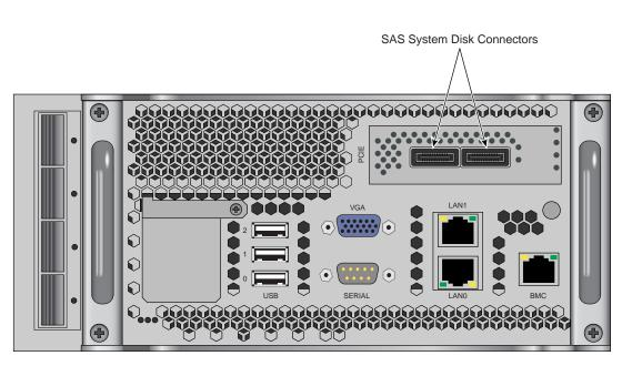
Figure 1-9 BaseIO Blade and PCIe Disk Controller Example
