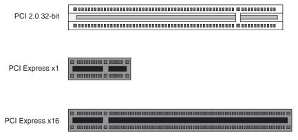
Figure 6-1 Comparison of PCI/PCI-X Connector with PCI Express Connectors
