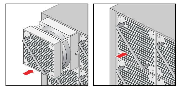
Figure 6-8Replacing an Enclosure Fan
