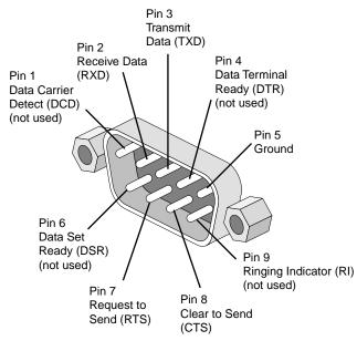
Figure A-3Serial Port Connector
