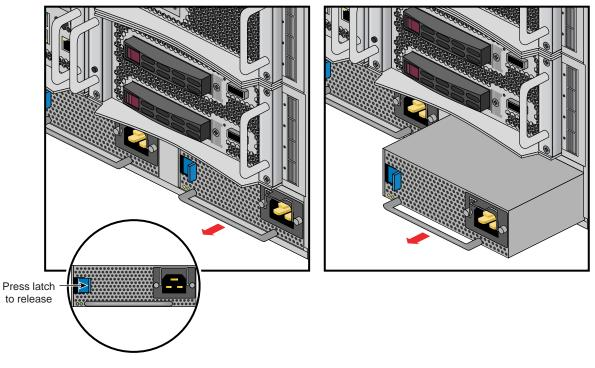
Figure 6-4 Removing an Enclosure Power Supply
