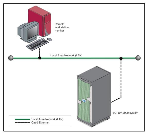
Figure 2-2 SGI UV 2000 LAN-attached System Control Network Example
