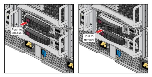
Figure 6-9 Removing the UV 2000 System Disk Example
