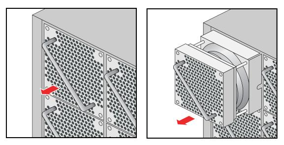
**Figure 6-7** Removing a Fan From the Rear Assembly
