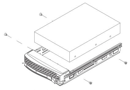
Figure 4-3Drive Carrier Mounting Example
