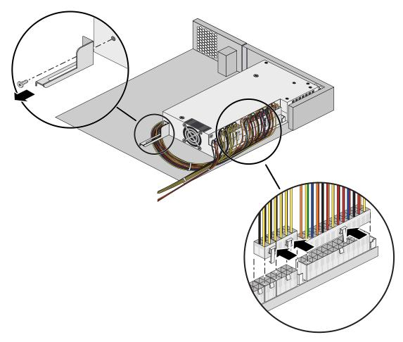
Figure 4-10 Removing the 450-Watt Non-Redundant Power Supply
