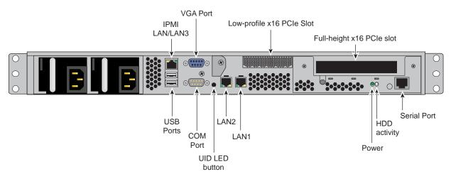
Figure 3-1 Server Rear Connectors Example
