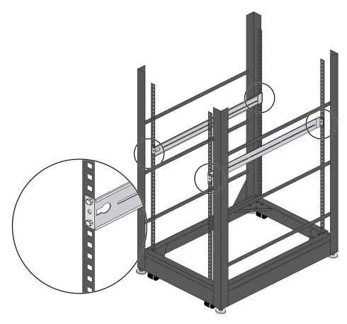
Figure 2-3 Outer Rail Attachment to Rack Example
