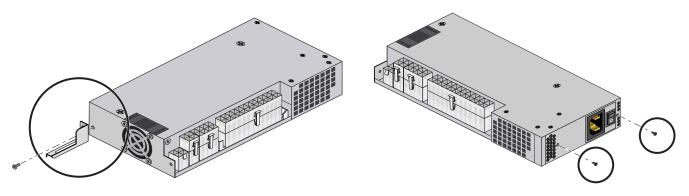
Figure 4-11450-Watt Power Supply Replacement Example
