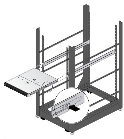
Figure 2-4 Sliding the System into a Rack
