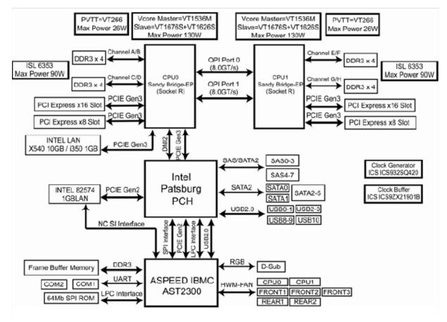
Figure 1-3 Functional Block Diagram of SGI Rackable C1110-RP6 System Server Board
