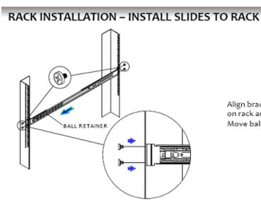
Align brackets to desired vertical position on rack and insert fasteners. Move ball retainer to the front of slides.
