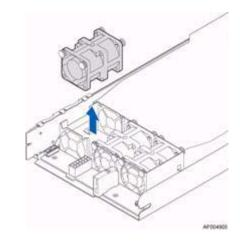
Figure 4-9Removing a Fan Set
