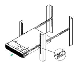
Fully extend the slides until it is in the locked position, pull the release button to release lock and disconnect inner member from slides.
