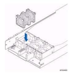
Figure 4-10 Installing a Fan Set
