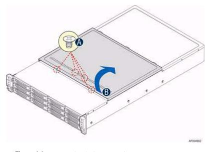
Figure 4-1Removing the System Top Cover
