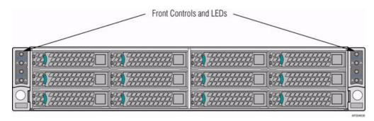
Figure 1-8 Front Control Panels
