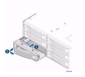
Figure 4-6 Inserting 3.5" HDD into Chassis
