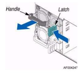
Figure 4-3Removing the Power Supply Unit
