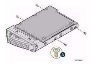
Figure 4-5Installing 3.5" HDD into Carrier
