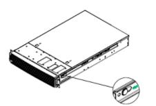
Align inner member key holes to standoffs on chassis, move inner member following the direction in left pictures.
