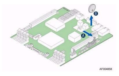
Figure 4-11Replacing the Backup Battery
