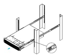
Pull the release button in the inner member to release the lock and allow the chassis to close.
