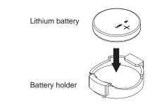
Figure 2-1 Installing the Onboard Battery
