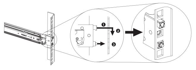
Figure C-1 Attaching Rail Slides to Rack
