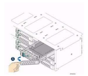
Figure 4-8 Inserting 2.5" HDD into Chassis
