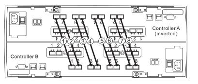
Paths 5, 7, 2, 4, 6, and 8 are used (in that order) to connect drive trays 3 through 8. You can connect up to 28 FC4600 drive trays, but the pattern changes after you connect eight drive trays. For detailed information, refer to the Hardware Cabling Guide.
