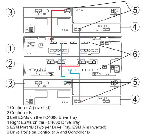
Adding a drive tray continues with the preceding pattern, with controller A using drive port 6 and controller B using drive port 3.
