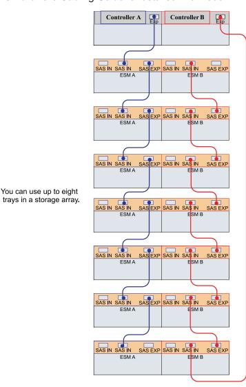
You can connect up to eight total trays for a maximum of 192 drives, including the 12 drives in the E2612 controller-drive tray.
