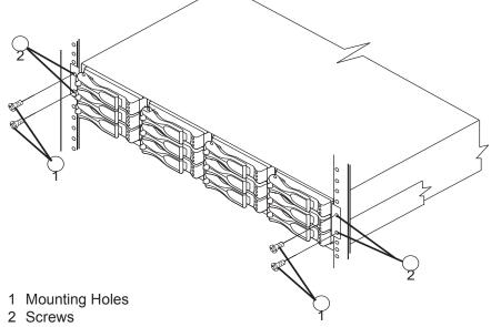
Secure the rear of the controller-drive tray to the cabinet by using two screws to attach the f langes on each side at the rear of the controllerdrive tray to the mounting rails.
