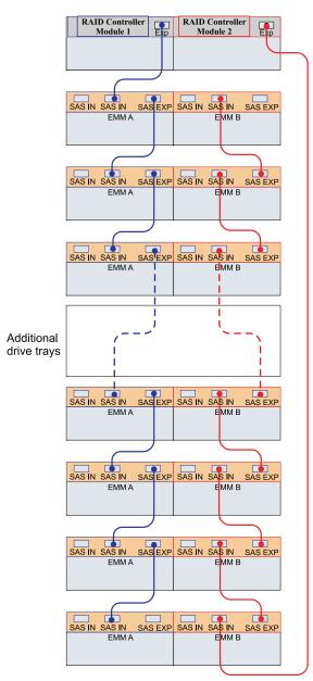
You can connect a combination of drive trays for a maximum of 384 drives, including the 12 drives in the E5412 controller-drive tray. You must also observe the 16-tray limit in all configurations.
