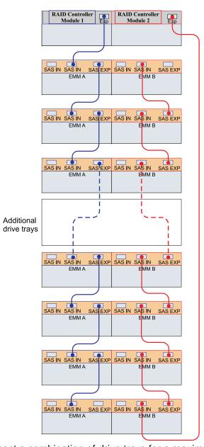
You can connect a combination of drive trays for a maximum of 384 drives, including the 24 drives in the E5424 controller-drive tray. You must also observe the 16-tray limit in all configurations.
