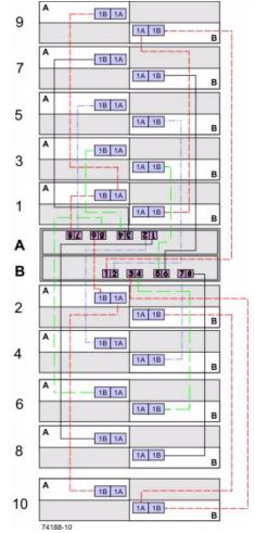
Figure 18 One CE7922 Controller Tray or CE7900 Controller Tray and 10 Drive Trays
