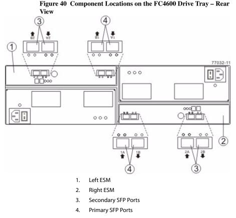
The ESM on the FC4600 drive tray has four SFP ports. The two primary ports are active. The secondary ports are reserved for future use. If SFP transceivers are placed in the secondary ports, the SFP Port LEDs blink, as a reminder that these ports are not functioning.
