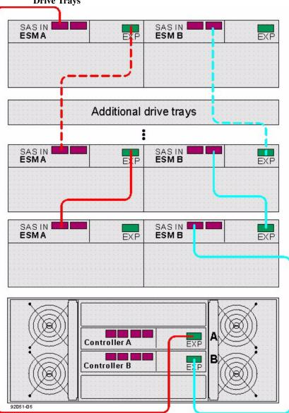
Figure 52 One E5460 Controller-Drive Tray and Seven or More Drive Trays
