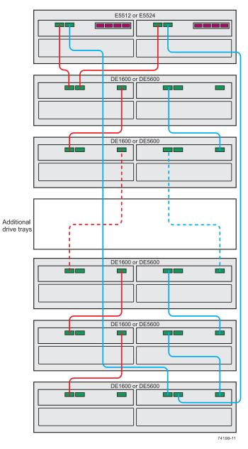
Figure 34 One E5524 Controller-Drive Tray or E5512 Controller-Drive Tray and up to 15 Drive Trays
