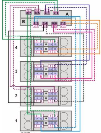
Figure 24 One CE7922 Controller Tray or CE7900 Controller Tray and Four DE6900 Drive Trays with Drive-Side Trunking
