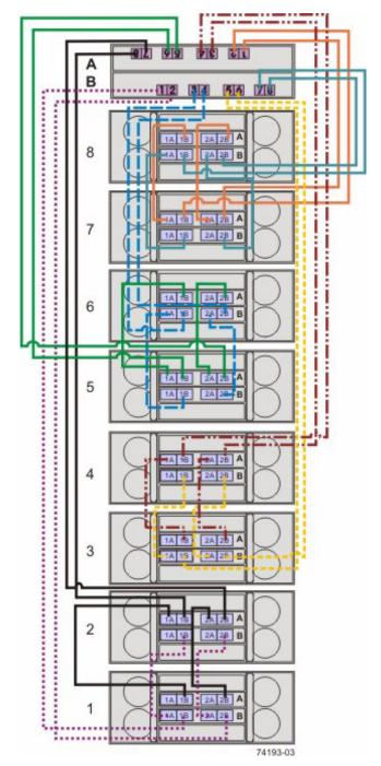
Figure 25 One CE7922 Controller Tray or CE7900 Controller Tray and Eight DE6900 Drive Trays with Drive-Side Trunking
