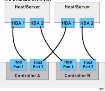
Figure 2 Direct-Attach Topology – Two Hosts and a Controller Tray or a Controller-Drive Tray
