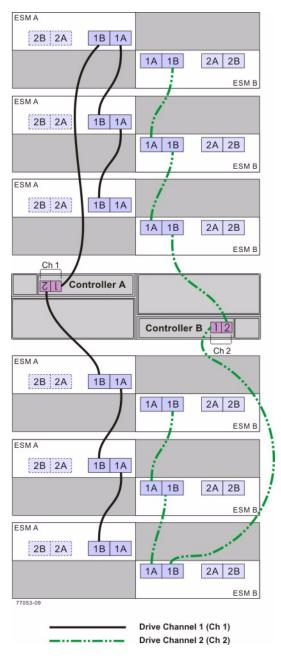
Figure 59 One CE4900 Controller-Drive Tray and Six FC4600 Drive Trays
