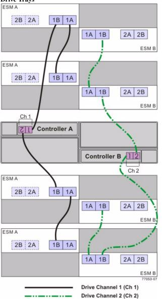
Figure 57 One CE4900 Controller-Drive Tray and Four FC4600 Drive Trays
