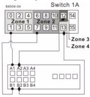
Figure 11 Storage Array Connections to Fibre Channel Switches
