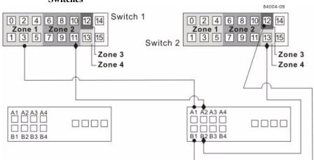
Figure 18 Secondary Storage Array Connections to Fibre Channel Switches
