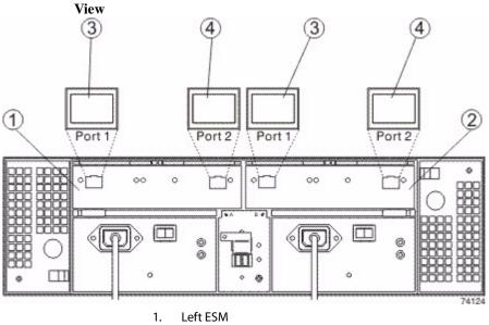
Figure 42 Component Locations on the FC2610 Drive Tray – Rear
