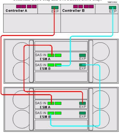
Figure 44 One E5424 Controller-Drive Tray or E5412 Controller-Drive Tray and Two DE6600 Drive Trays
