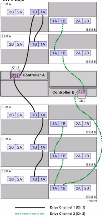
Figure 58 One CE4900 Controller-Drive Tray and Five FC4600 Drive Trays
