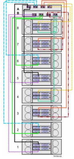
Figure 21 One CE7922 Controller Tray CE7900 Controller Tray and Eight DE6900 Drive Trays without Trunking
