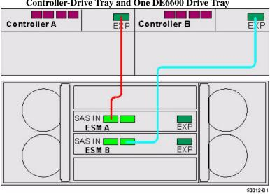
Figure 43 One E5424 Controller-Drive Tray or E5412 Controller-Drive Tray and One DE6600 Drive Tray
