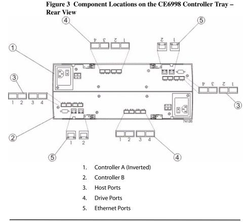
**NOTE** If you use remote mirroring, host port 4 on each controller of the CE6998 controller tray is reserved for that feature. If you do not use the remote mirroring feature, these host ports are available for host connections.
