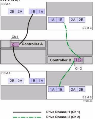
Figure 55 One CE4900 Controller-Drive Tray and Two FC4600 Drive Trays
