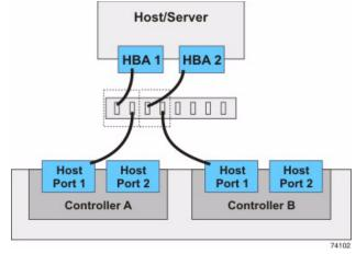
Two Hosts to a Controller Tray or a Controller-Drive Tray
