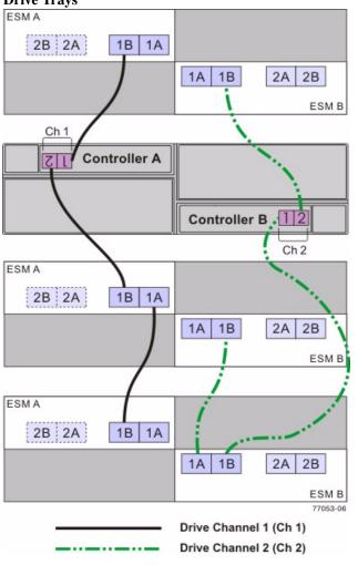
Figure 56 One CE4900 Controller-Drive Tray and Three FC4600 Drive Trays
