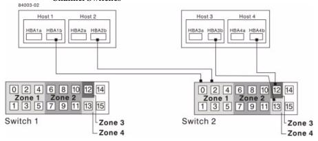
6. Connect controller port A1 of the primary storage array to an available port in zone 1 of switch 1.
