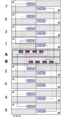
Note how the controller tray (denoted by A and B in the figure) is conveniently situated in the middle of the arrangement, which enables you to use cables that are all the same length. Positioning the controller tray near the middle of the cabinet also helps prevent the cabinet from becoming top heavy as drive trays are added.
