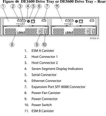
Figure 46 DE1600 Drive Tray or DE5600 Drive Tray – Rear View
