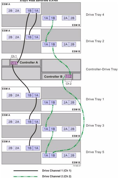
Figure 64 One CDE3994 Controller-Drive Tray and Five Drive Trays with Inverted ESMs
