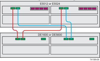
Figure 33 One E5524 Controller-Drive Tray or E5512 Controller-Drive Tray and Three Drive Trays
