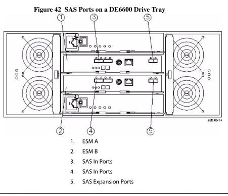
**WARNING** (W15) **Risk of bodily injury** – An empty tray weighs approximately 56.7 kg (125 lb). Three persons are required to safely move an empty tray. If the tray is populated with components, a mechanized lift is required to safely move the tray.
