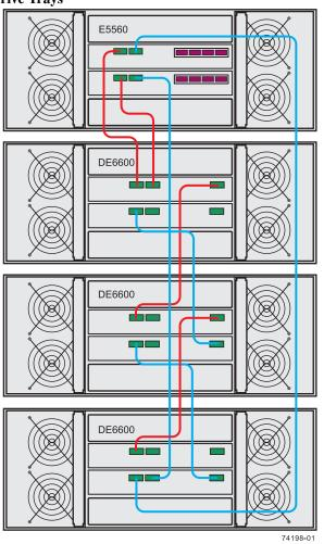
Figure 37 One E5560 Controller-Drive Tray and Three DE6600 Drive Trays
