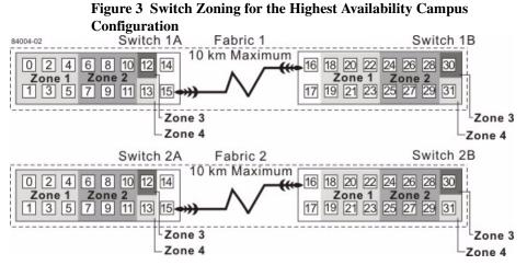
Before you proceed, review the requirements listed in this section and the zoning shown in the figure to make sure that all four switches are correctly zoned. For more information, see the Fibre Channel Configurations Overview.
