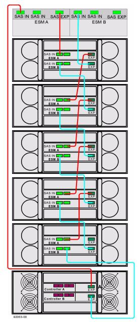
Figure 53 A Storage Array with the Capacity for 384 Drives Using a E5460 Controller-Drive Tray
