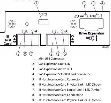
Figure 19 E5400 Right-Rear Subplate with an InfiniBand Host Interface Card
