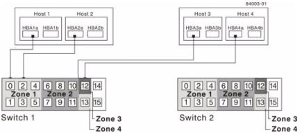
5. Connect the secondary host bus adapter for each host to an available port in zone 1 of switch 2.
