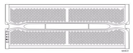
Figure 38 DE6600 Drive Tray – Front View with the Bezel Removed
