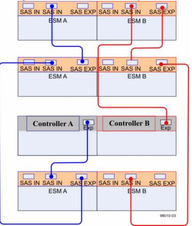
Figure 70 One E2600 Controller-Drive Tray and Three Drive Trays
