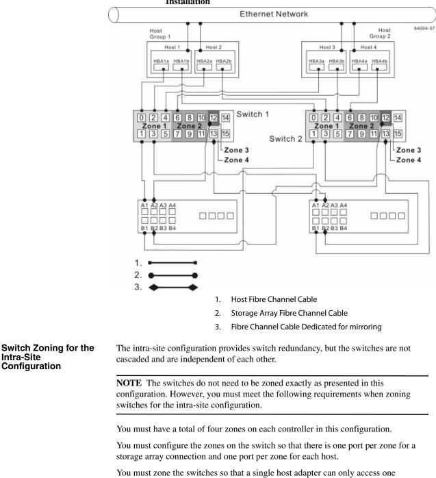
Figure 13 Intra-Site Configuration Following a Complete Installation
