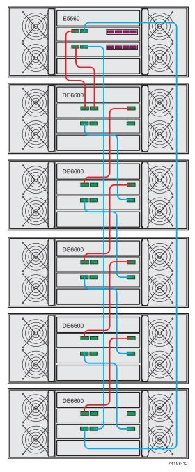
The figures above show storage arrays with DE6600 drive trays. A storage array with an E5560 controller-drive tray might also include DE1600 drive trays or DE5600
