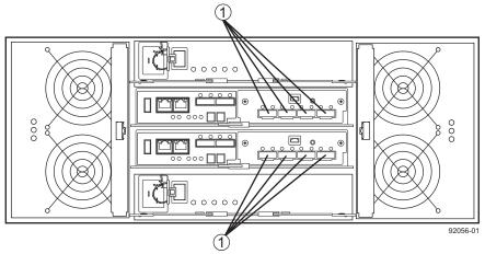
Figure 5 Host Channels on the E5560 Controllers with SAS HIC – Rear View92056
