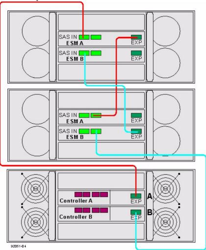
Figure 51 One E5460 Controller-Drive Tray and Two DE6600 Drive Trays
