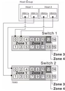
Figure 4 Host Bus Adapter Connections to Fibre Channel Switches
