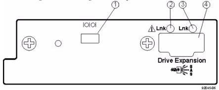
Figure 17 E5400 Right-Rear Subplate with No Host Interface Card
