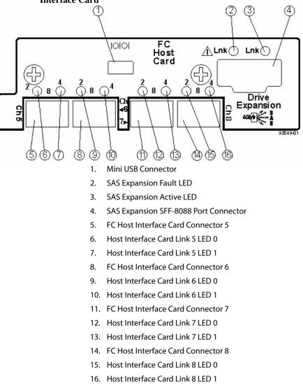
Figure 18 E5400 Right-Rear Subplate with an Fibre Channel Host Interface Card
