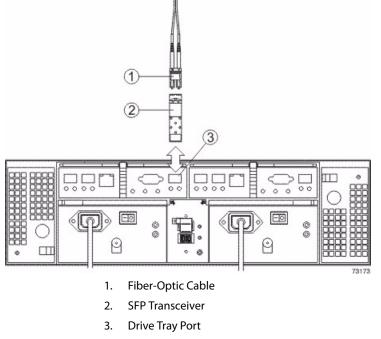
4. Install the fiber-optic cable.
