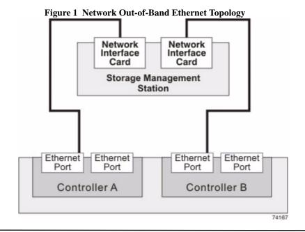
**NOTE** In limited situations where the storage management station is connected directly to the controller tray or the controller-drive tray, you must use an Ethernet crossover cable to connect the storage management station to the Ethernet port. An Ethernet crossover cable is a special cable that reverses the pin contacts between the two ends of the cable.
