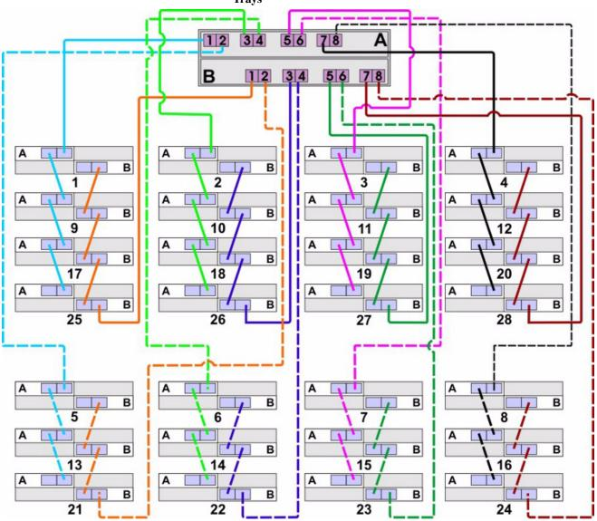
Figure 19 One CE7922 or CE7900 Controller Tray and 28 Drive Trays
