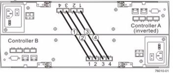
Table 2 Redundant Path Pairs on the CE6998 Controller Tray
