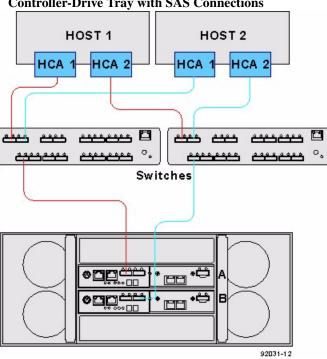
Figure 8 Switch Topology – Two Hosts and a E2660 Controller-Drive Tray with SAS Connections
