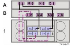
Figure 23 One CE7922 Controller Tray or CE7900 Controller Tray and Two DE6900 Drive Trays with Drive-Side Trunking
