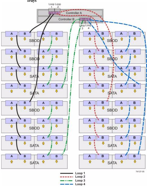
Figure 30 One CE6998 Controller Tray and Multiple Types of Drive Trays
