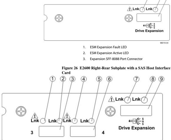
Figure 25 E2600 Right-Rear Subplate with No Host Interface Card
