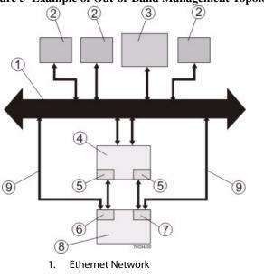
Figure 5 Example of Out-of-Band Management Topology
