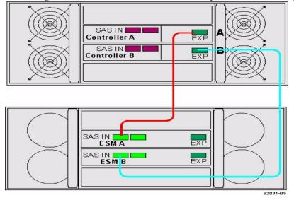
Figure 74 One E2660 Controller-Drive Tray and Two Drive Trays
