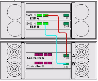
Figure 50 One E5460 Controller-Drive Tray and One DE6600 Drive Tray
