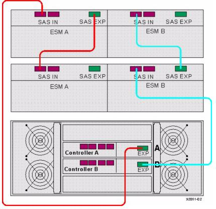
Figure 48 One E5460 Controller-Drive Tray and Two DE1600 Drive Trays or DE5600 Drive Trays
