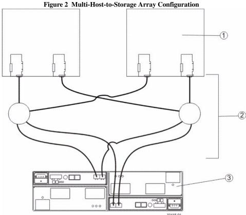
Two Host Systems, Each with Two Fibre Channel Host Bus Adapters
