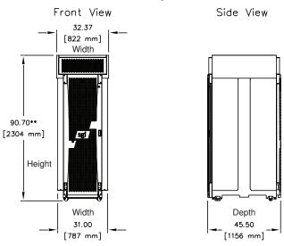
\*\*Rack height can be reduced to 78.75 in (2000 mm) for shipping.
