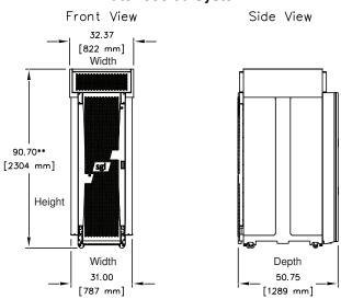
Figure 3-4 SGI UV 2000 Compute Rack Dimensions (Routered Configurations)
