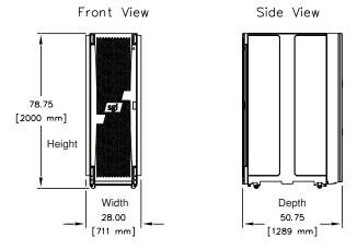
Figure 3-3 SGI UV 2000 Compute Rack Dimensions (Routerless Configurations)
