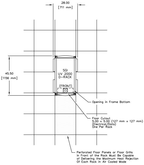
**Note**: Equipment shown on 24 inch floor tile Approximate area of 10 square feet (0.9 square meters) without access Approximate area of 30 square feet (2.8 square meters) with access
