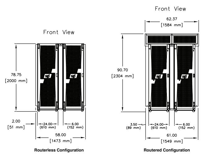
Note: The dimensions shown in this figure are valid for both air-cooled configurations and water-cooled configurations.
