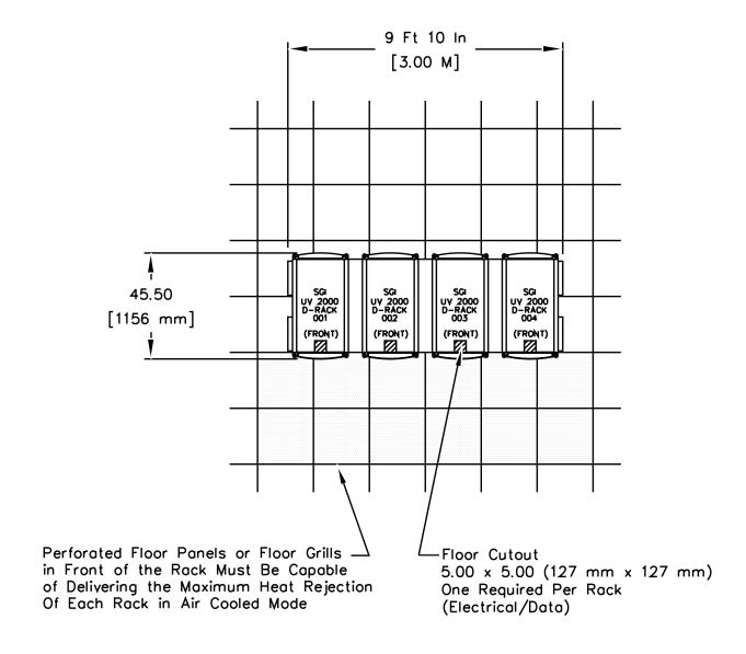
Figure 4-2 Four Air-cooled Racks Floor Layout (Shown on 24-in by 24-in Grid)
