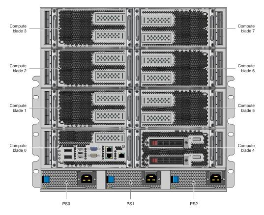
Figure 2-3 IRU Components - Front
