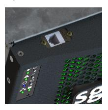
Figure 1-76 MIS-S9D Proprietary Network Interface
