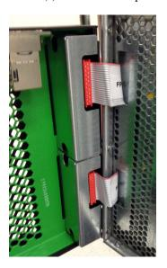
Figure 1-4 Control Panel Ribbon Cables Attached to Front Bezel
