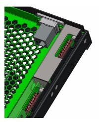
**Figure 1-2** Front Bezel Grille Control Panel Sockets and S9D Network Interface
