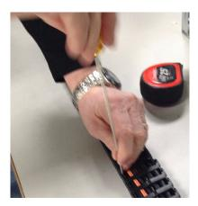
Figure 1-53 Pry Open the Segment Joint
