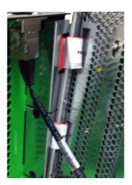
Figure 1-5 S9D Network Interface Cable
