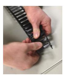
**Figure 1-50** Pull the Segments from the Arm
