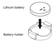
Figure 2-1 Installing the Onboard Battery
