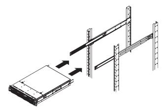
Figure 3-3 Installing the Server in a Rack
