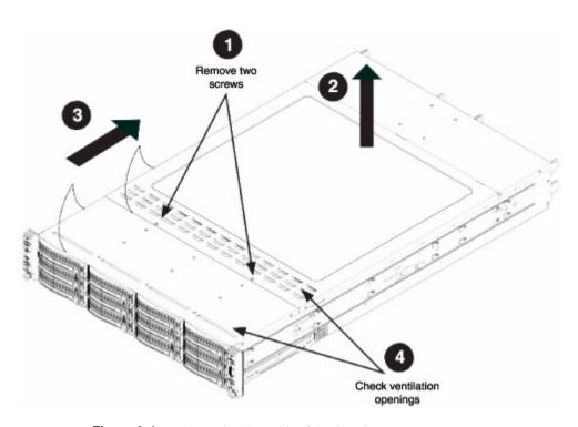
Figure 3-4 Accessing the Inside of the Chassis
