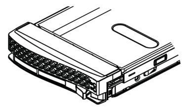
**Figure 5-5** Drive Carrier Release Tab
