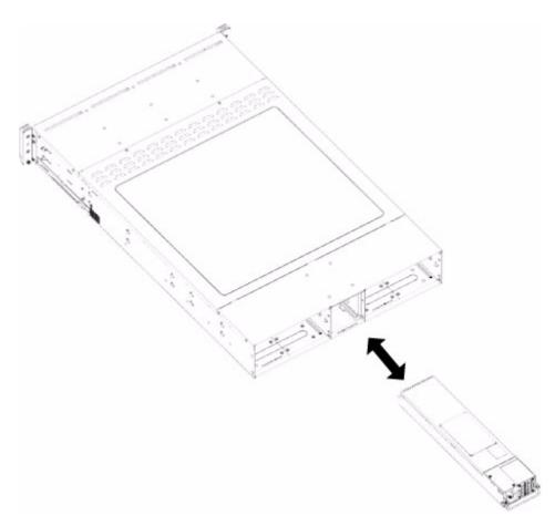
**Figure 5-3** Removing the Power Supply
