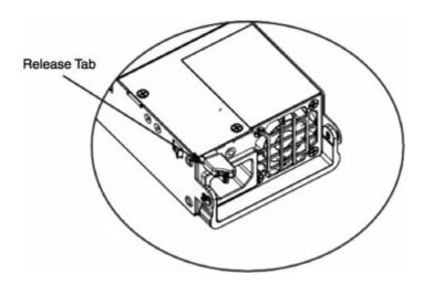
Figure 5-2 Power Supply Release Tab
