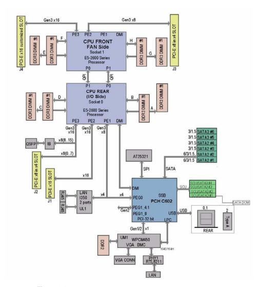
Figure 1-4 Serverboard Block Diagram
