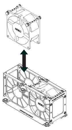
Figure 5-9 Removing Fan from Fan Housing
