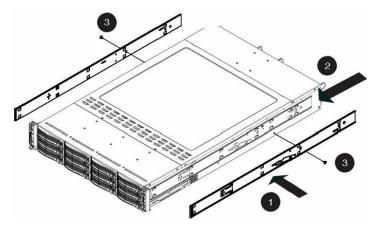
Figure 3-2 Installing the Inner Rail Extensions
