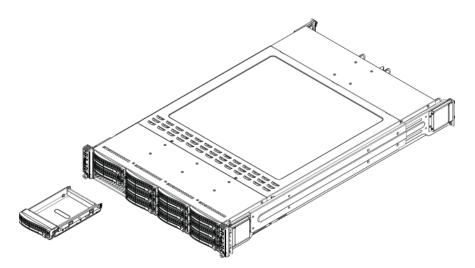
**Figure 5-6** Removing Drive Carrier From Chassis
