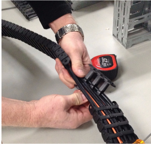
Figure 26 Twist the Section of Segments from the Cables
