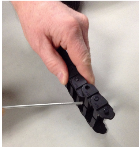
Figure 19 Pry the Joint Apart
