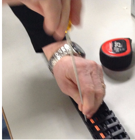
Figure 23 Pry Open the Segment Joint
