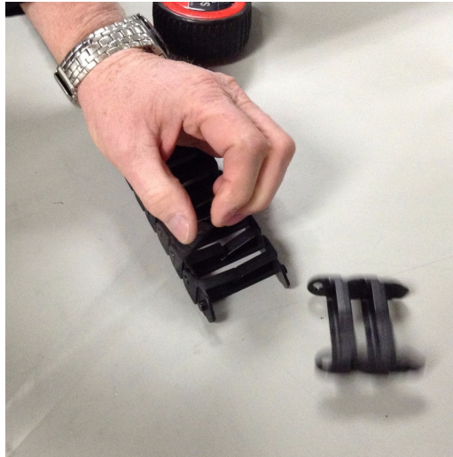
Figure 21 Shortened Arm Ready for Installation
