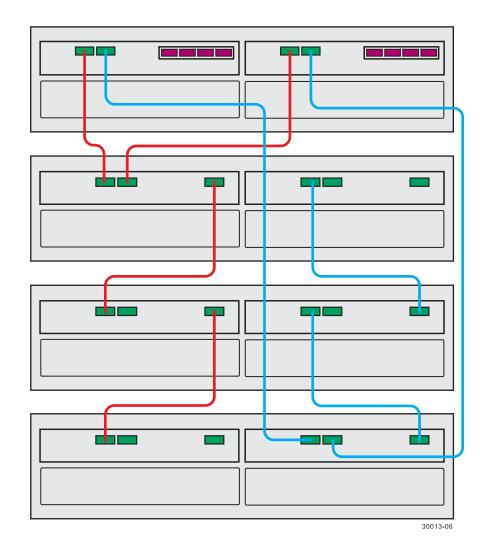
Steps to connect Ethernet cables for out-of-band management only:
