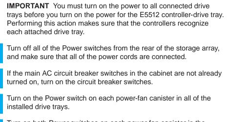
Turn on both Power switches on each power-fan canister in the E5512 controller-drive tray.
