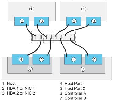
Attach the cables to the drive trays as needed. For maximum redundancy and tray loss protection, see the following figure.
