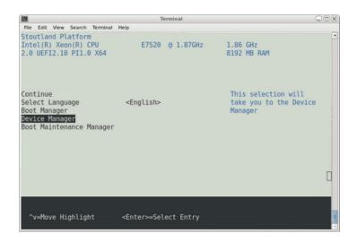
Figure 2-8 SGI UV 2000, SGI UV 1000, or SGI UV 100 Boot Manager Screen
