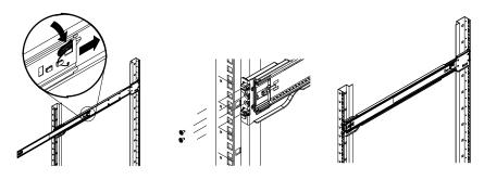
Figure 2-3 Outer Rack Rail Assembly/Placement Example
