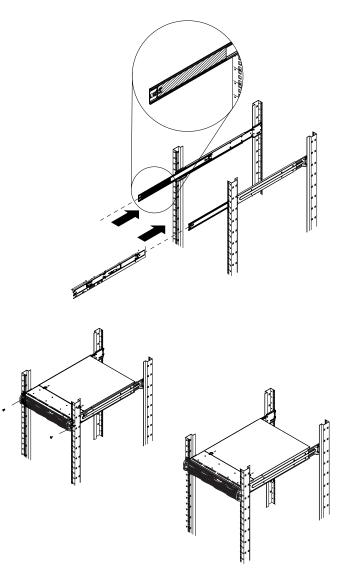
Figure 2-5 Installing the Server in the Rack
