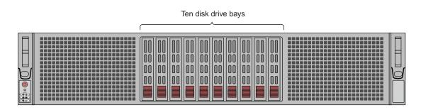
Figure 5-3 C2110G-RP5-P System Disk Drive Locations
