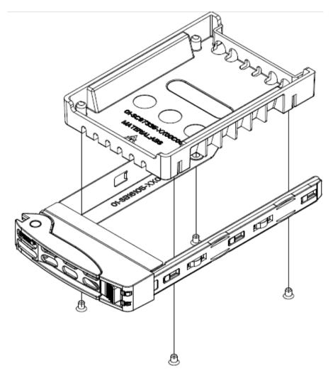
Figure 6-2 Drive Carrier Attachment to Dummy Drive Blank
