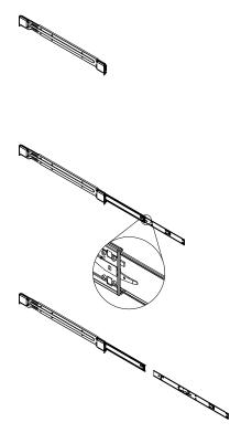
Figure 2-2 Separating the Rack Rails
