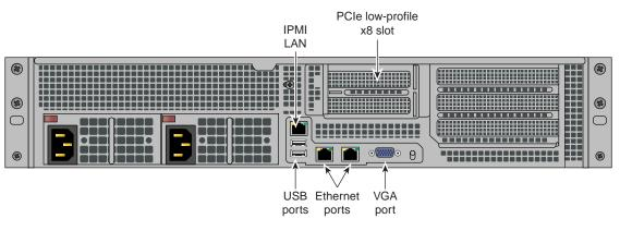
Figure 6-10 Low-Profile PCIe Slot Location
