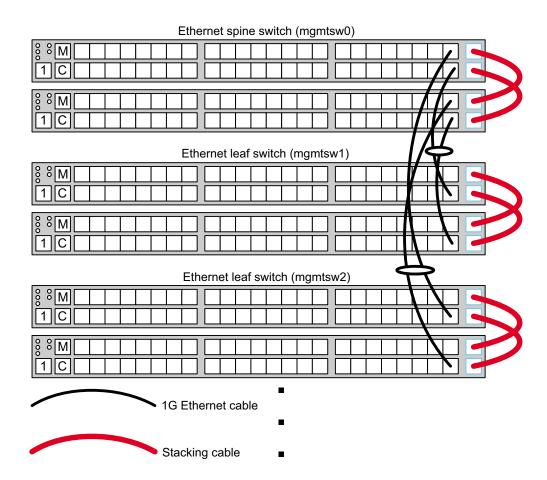
Figure B-1 Spine Switch and Leaf Switches
