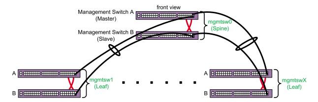
Figure 3-11 Switch Stack With Multiple Switches
