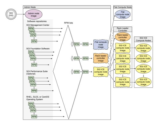
Figure 3-1 SGI Management Center Software Installation Process
