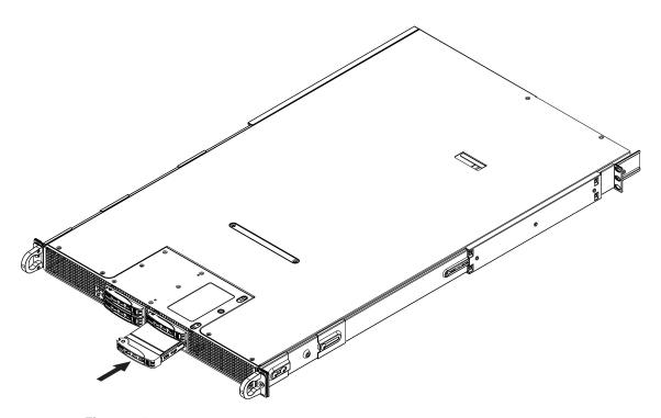
Figure 6-4 Hard Disk Drive Installation Example
