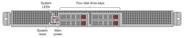
Figure 5-3 C1104-GP1 System Disk Drive Locations
