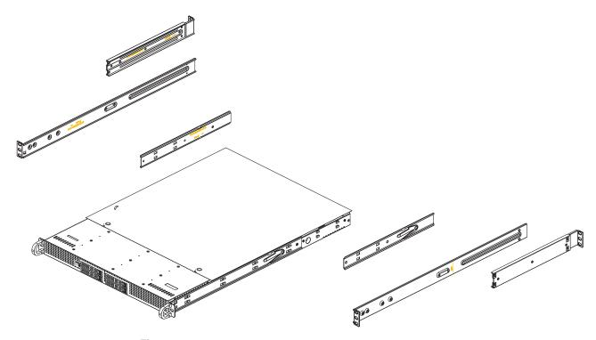
Figure 2-2 Separating the System Rack Rail Components
