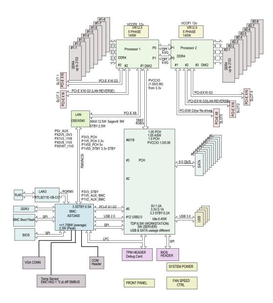
Figure 1-2 Processor, Memory and I/O Chipset System Block Diagram
