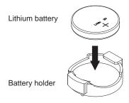
Figure 4-1 Installing the Onboard Battery
