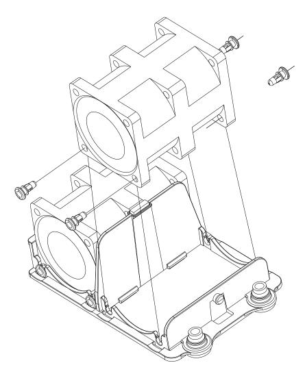
Figure 6-8 Individual Fan Remove/Replace Example
