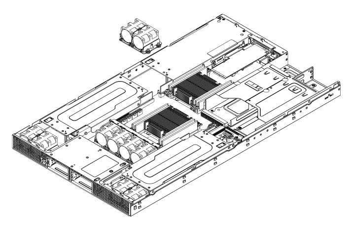
Figure 6-7 Remove/Replace Fan Assembly Example
