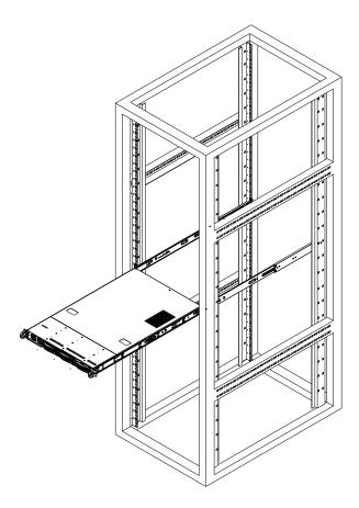
Figure 2-6 Installing the Server in the Rack
