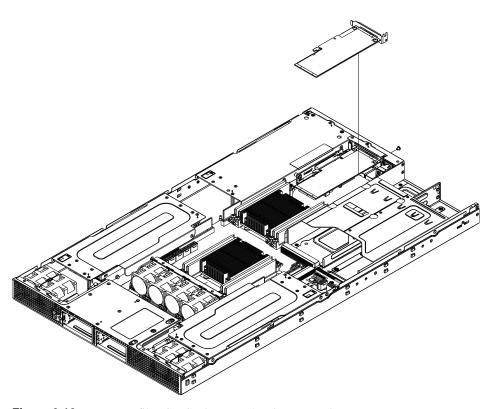
Figure 6-10 Low-profile PCIe Card Remove/Replace Example
