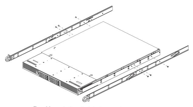
Figure 2-3 Rail to Server Chassis Attachment Example
