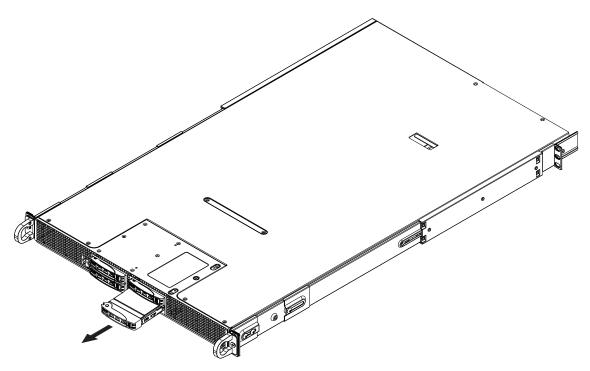
**Figure 6-2** Remove Drive and Carrier from Front of Server
