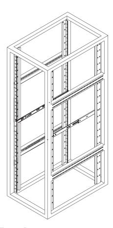
Figure 2-5 Outer Rack Rail Assembly/Placement Example
