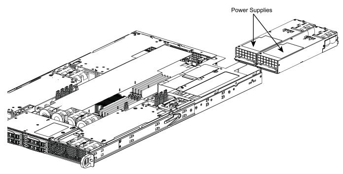
Figure 6-5 Power Supply Remove/Replace Example
