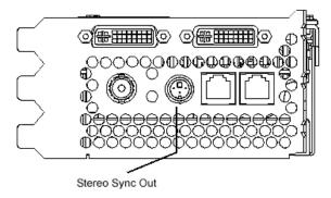
Figure 7. Stereo Sync Out Port (Shown On Wildcat 4210)
