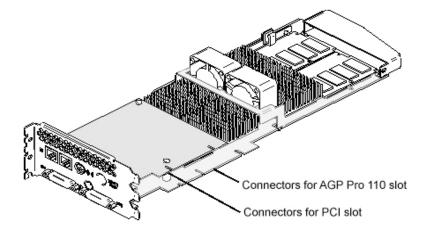
Figure 4. Expansion Slot Connectors (Shown On Wildcat 4210)
