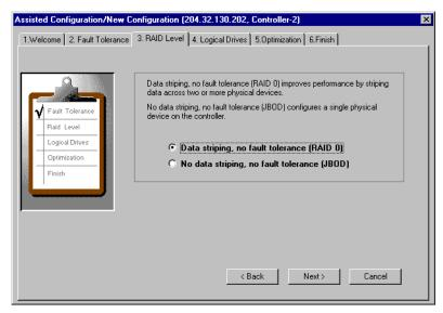
Figure 4-39. Assisted Configuration - RAID Level With No Fault Tolerance
