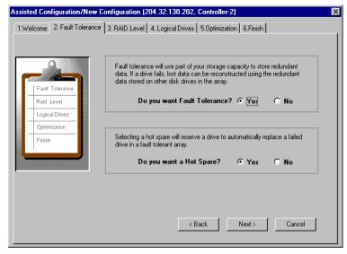
Figure 4-37. Assisted Configuration - Fault Tolerance
