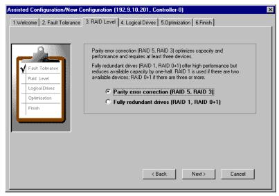
Figure 4-38. Assisted Configuration - RAID Level With Fault Tolerance
