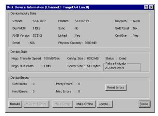
Figure 6-2. Rebuild Button Available for This Disk Device
