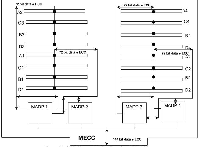
Figure 4-2: SKA4 Memory Module Functional Block Diagram
