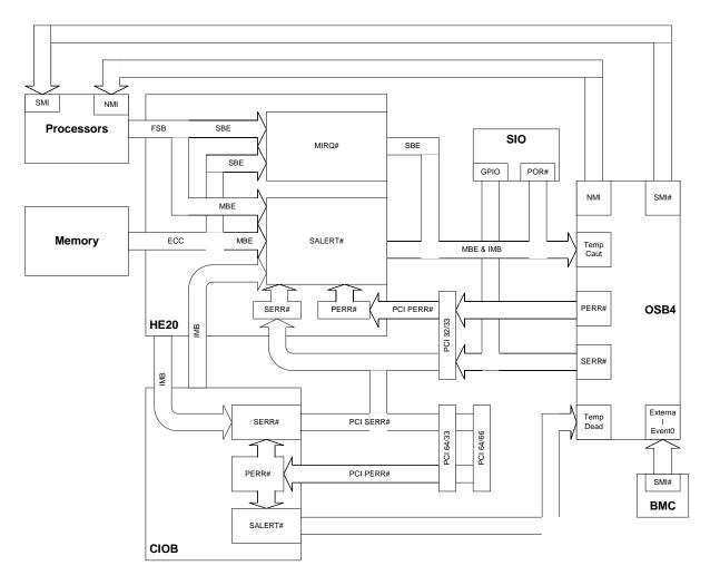
Figure 7-1: SKA4 Error Signal Propagation to SMI#
