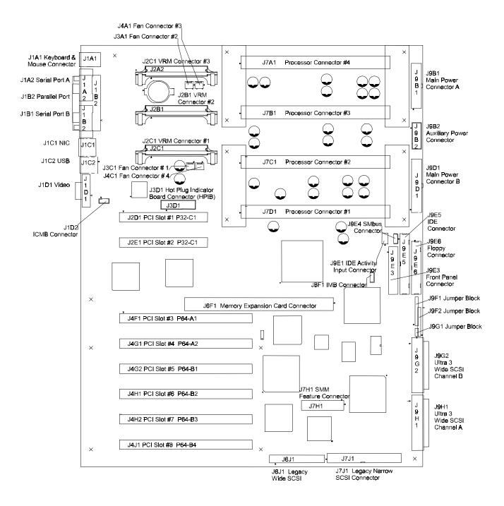
Figure 11-1: SKA4 Baseboard Connector Identification and Locations
