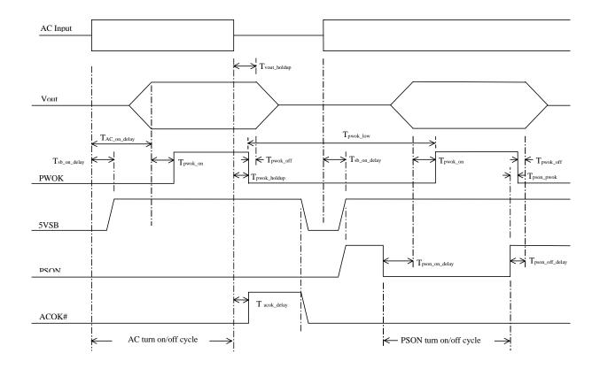
Figure 12-2: Turn On/Off Timing
