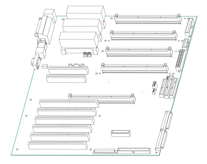
Figure 1-2: SKA4 MP Baseboard Layout Diagram
