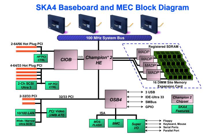
Figure 1-1: SKA4 MP Server Functional Block Architecture
