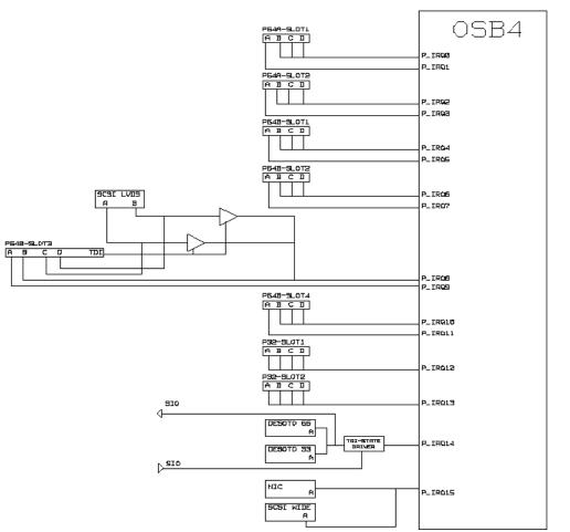
Figure 2-1: SKA4 Baseboard Interrupt Diagram
