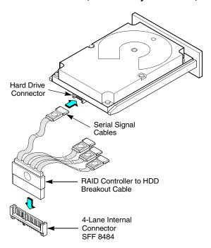
Figure 2.3 displays the SATA II device plug connector that connects a SAS RAID controller with internal connectors to the host receptable connector on a backplane. A SATA II connector consists of a signal connector and a power connector.
