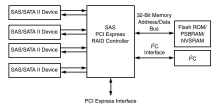
Figure 1.2 shows an example of a SAS RAID controller configured with an LSISASx12 expander that is connected to SAS disks, SATA II disks, or both.
