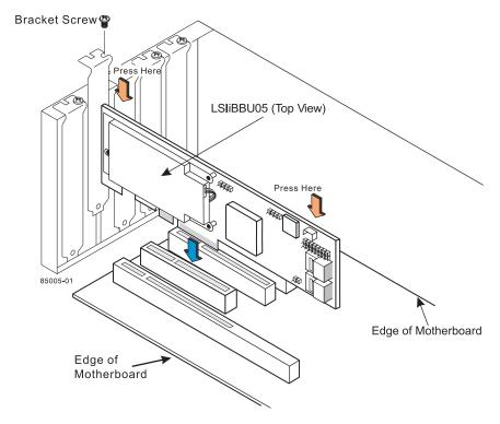
Step 6. Configure and Install the SAS Devices, SATA II Devices, or Both in the Host Computer Case
