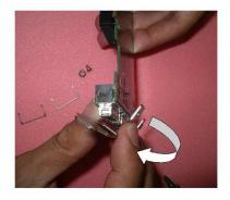
(c) Rotate the bracket toward the Component Side.
