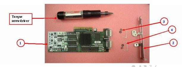
**Step 1 - Place short bracket onto card** 5. Gently place the bracket onto the card fitting the connectors through the bracket connector holes. Make sure the LEDs are aligned into their intended bracket holes. **Step 2 - Attach**
