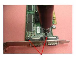
Figure 10: Unscrew Bracket Screws
