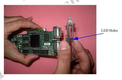
**short bracket to card**Insert a screw along with a washer into each of the two holes on the card intended for holding the bracket. Use a torque screwdriver to apply up to 2 lbs-in torque on each screw.
