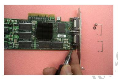
**Step 3 - Install Connector Clips** 1.Gently push one clip onto the connector. Make sure to slide both clip hooks (sides) around the connector evenly as shown in Figure 18.
