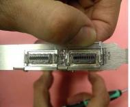
2. Use a small flat head screwdriver to gently slide the clip's hook towards the connector's base side as shown in Figure 19.
