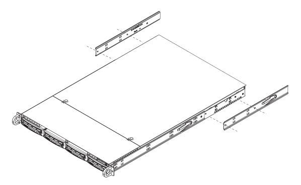
Figure 2-2. Installing the Rack Rails
