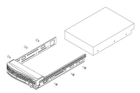
Figure 6-4. Mounting a Hard Drive in a Carrier
