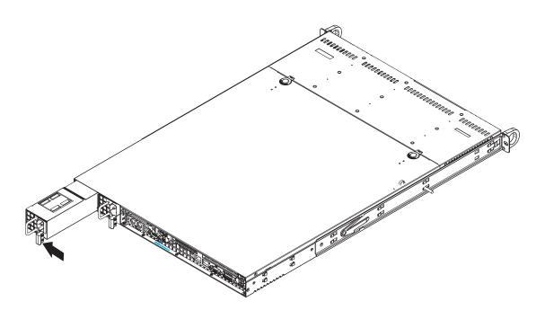
Figure 6-6. Removing/Replacing the Power Supply
