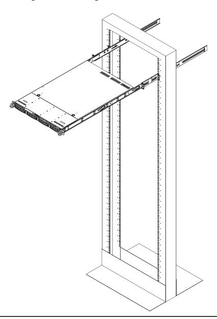
Figure 2-4. Installing the Server into a Telco Rack
