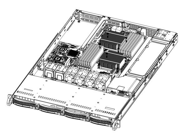
Figure 6-2. System Cooling Fans
